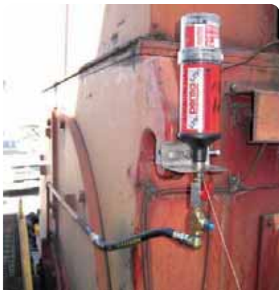
Lubricator: perma Star Vario Bracket: MB01 with BC65 Install Kit: K165 Ref #: MOTOR07
