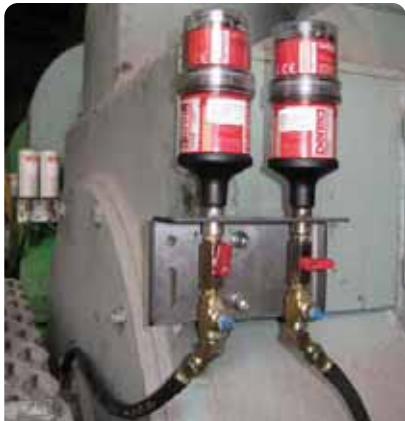
Lubricator: perma Star Vario Bracket: MB02-R with BC65 Install Kit: K2RR (modified) Ref #: MOTOR04
