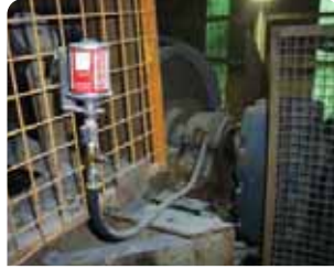
Remote installed perma Classic utilising the CH01-S stainless steel bracket.
