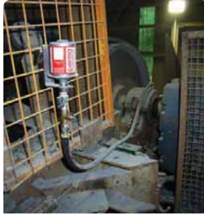
Lubricator: perma Classic Bracket: CH01-S Install Kit: K1CH100 Ref #: CONV02
