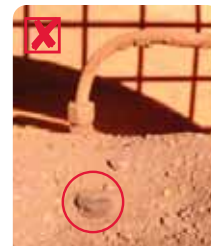
Poor manual greasing practises lead to contamination and a reduction in bearing service life. WHERE POSSIBLE FIT COVERS TO GREASE NIPPLES.
