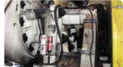
Equipment: Warman pump perma Star Vario MB02-C with BC65 Lubricator: perma Star Vario MB02-C with BC65 Bracket: K265C Install Kit: K265C Ref #: PUMP09
