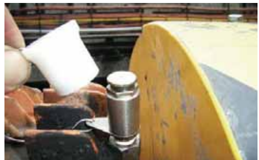
*The sample shown is for a 1/4" BSP greasing port and has a button head type nipple.
