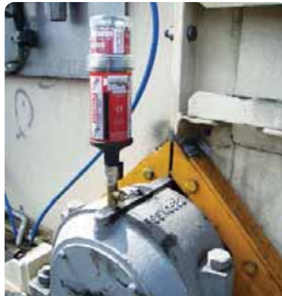
Lubricator: perma Star Vario Bracket: Direct Ref #: CONV07
