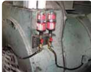
Remote installed perma Star Vario using a 2-point stainless steel bracket.
