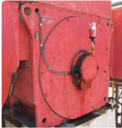
Lubricator: perma Star Vario Bracket: Direct Ref #: MOTOR02
