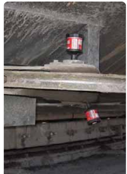
Lubricator: perma Futura Equipment: Wire rope sheaves Bracket: Direct Ref #: OTHER04
