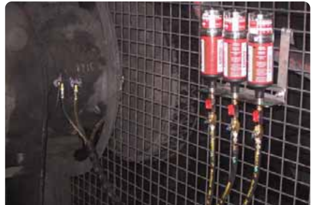
Lubricator: perma Star Vario Bracket: CH03 Install Kit: K3CH Ref #: CONV05
