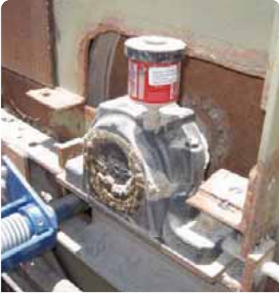
Lubricator: perma Futura Bracket: Direct Ref #: CONV01
