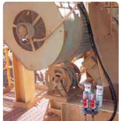
Lubricator: perma Star Vario Bracket: MB02-C with BC30 Install Kit: K230C Ref #: MOTOR09
