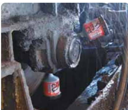
The harshest conditions occur when bearings are subjected to high levels of dirt and water. Direct mounted perma Futura's provide a positive purge of grease to protect this bearing.
