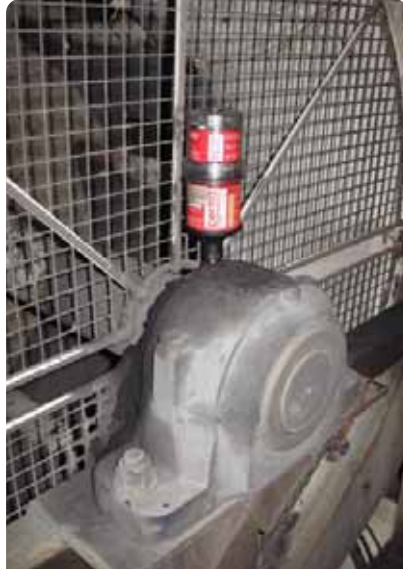
Lubricator: perma Star Vario Bracket: Direct Ref #: FAN03
