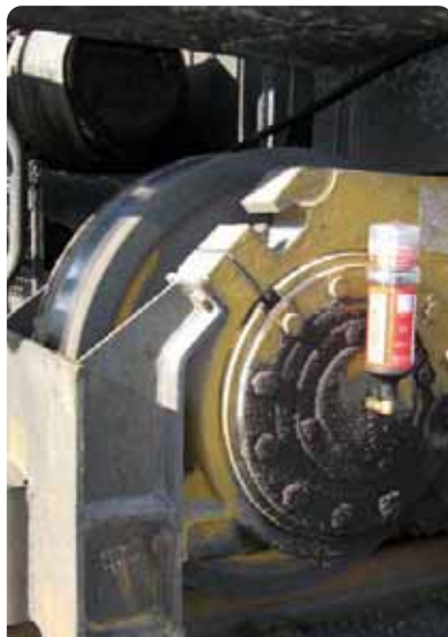
Lubricator: perma Star Vario Equipment: Overhead crane travel wheels Bracket: Direct Ref #: OTHER03
