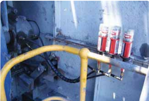
Lubricator: perma Star Vario Bracket: MB03 with BC30 Install Kit: K330 Ref #: CONV04
