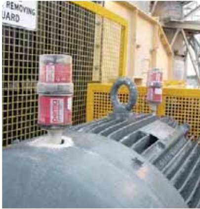
Lubricator: perma Star Vario Bracket: Direct Ref #: MOTOR01
