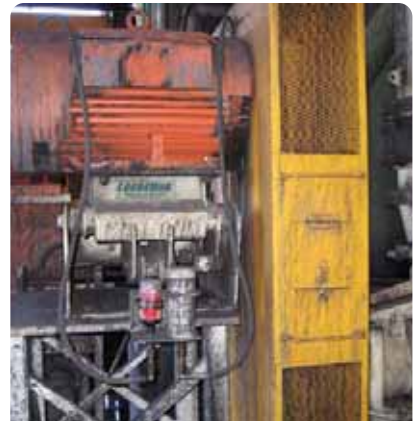
Lubricator: perma Star Vario Bracket: MB02-C with BC30 Install Kit: K230C Ref #: MOTOR06
