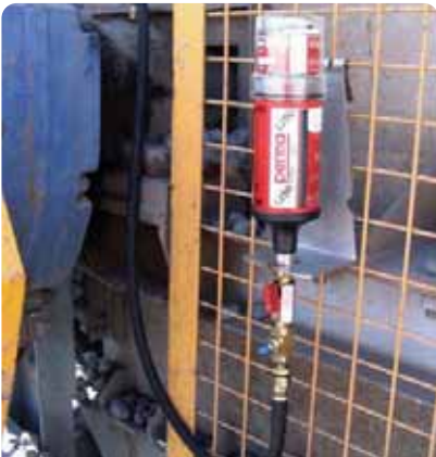
Lubricator: perma Star Vario Bracket: CH01 Install Kit: K1CH Ref #: CONV06
