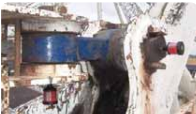
Lubricator: perma Futura Equipment: Wire rope pins & sockets Bracket: Direct Ref #: OTHER01
